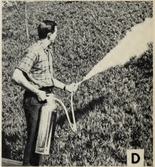
Fig. 28. Equipment used in "built-in pest control" at the time of construction of a building. A. electric blower for dusting attics via the attic "crawl hole"; B. dusting subcabinet voids; C. dusting wall voids; D. a fire extinguisher for blowing insecticide dust which may be used in place of the two other dusters shown in the figure.
